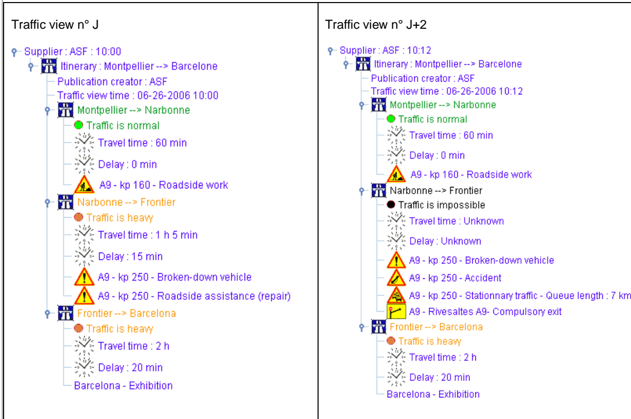
Example of traffic view display 3 (snapshot n° J and snapshot n° J+2)
