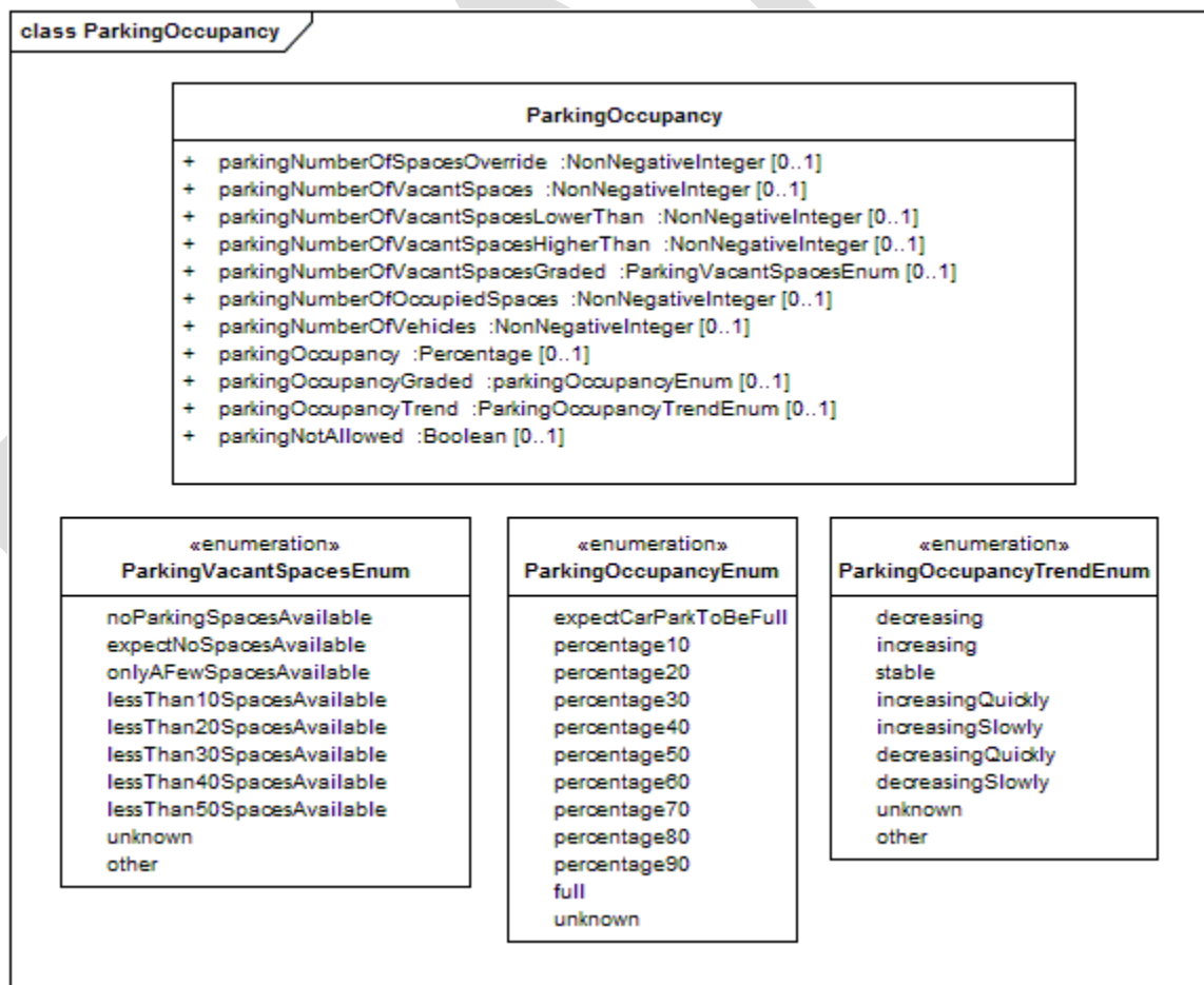
Figure C.5 — “ParkingOccupancy” with enumerations
